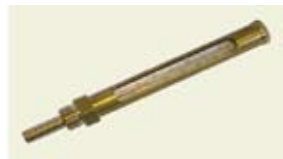
Flow water thermometer, to be positioned no more than 1 metre from the boiler, tapping 1/2 " male.
